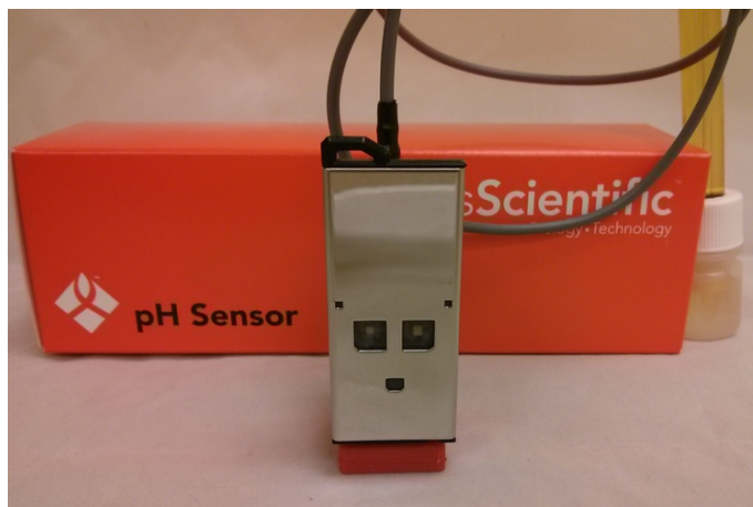
Figure 6: Setting up: Part 3. Plug the main housing into the Sensordrone (the Sensordrone should be facing out/away from the housing). Be sure your Sensordrone is charged up!
