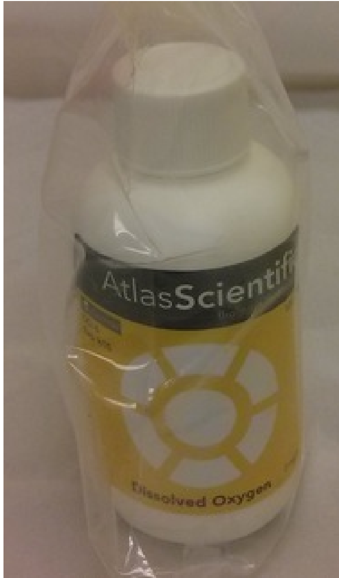
Figure 9: A 0-Dissolved Oxygen solution, used to confirm that the probe is properly working.
