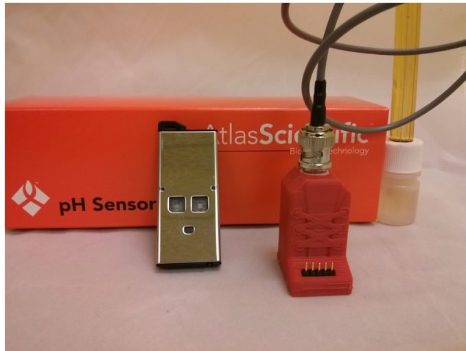
Figure 5: Setting up: Part 2. Attach the probe to the BNC connector on the main housing.
